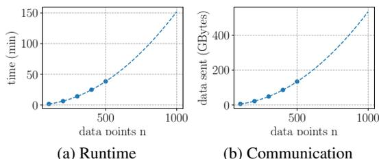
Figure 4: Efficiency benchmark per clustering iteration for privacy-preserving AP with 2 parties and passive security.
