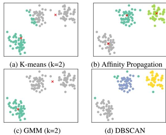
Figure 2: Effect of setting the wrong number of clusters  $k$  for clustering with k-means and GMM, whereas DBSCAN and AP determine the number of clusters automatically. The red crosses mark the clusters’ centroids in the respective clustering algorithm’s output.
